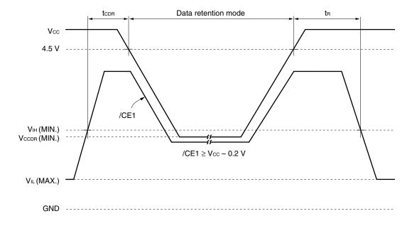
$\label{eq:Remark} \begin{array}{ll} \mbox{Premark} & \mbox{On the data retention mode by controlling /CE1, the input level of CE2 must be CE2 <math display="inline">\geq V_{CC}-0.2 \ V \ or \ CE2 \leq 0.2 \ V. \ The other pins (Address, I/O, /WE) can be in high impedance state. \end{array}$
