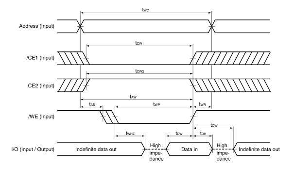
Cautions 1. During address transition, at least one of pins /CE1, CE2, /WE should be inactivated.2. When I/O pins are in the output state, therefore the input signals must not be applied to the output.
