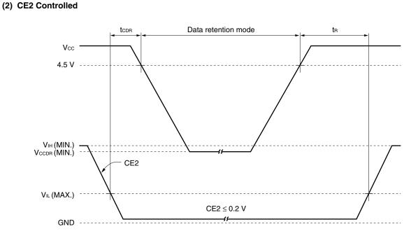
**Remark** On the data retention mode by controlling CE2, the other pins (/CE1, Address, I/O, /WE) can be in high impedance state.
